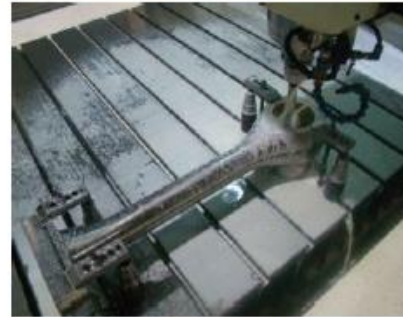
Connection rods repair
